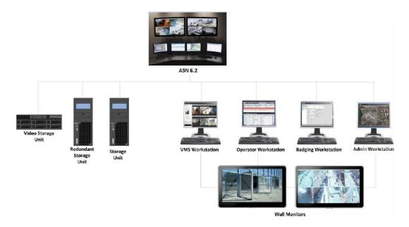
Additional workstations (Administrator's Workstation, Badging Workstation, etc.) can be networked into the system, per the diagram above.
